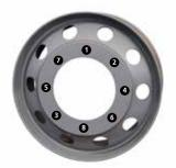
**2.** Fit and tighten the nuts with a calibrated torque wrench at the recommended torque, in the sequences illustrated here.
