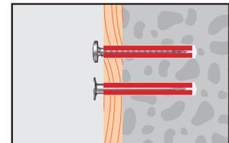
4. With fixture firmly held in place fasten with a 6 or 8 gauge screw or minimum 3.5mm nail.
