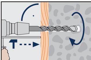
1. Drill 5.0-5.5mm diameter hole. Drill hole to required depth so that screw or nail can be driven home.
